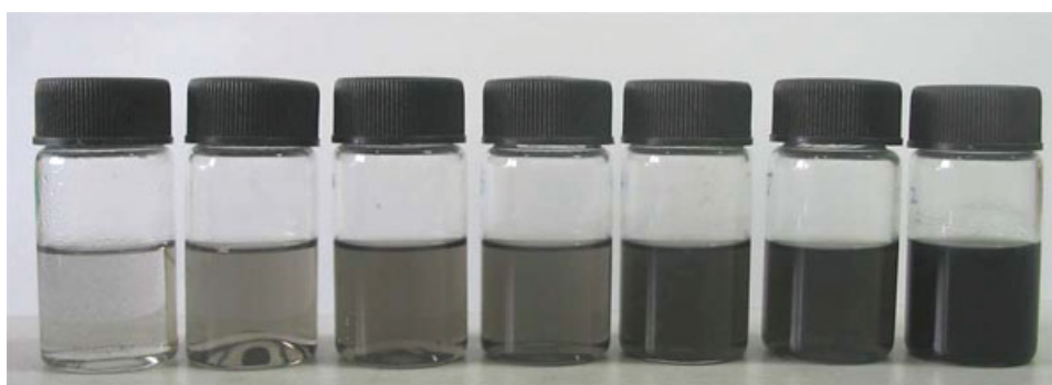
Figure 2 Photos of the supernatant solutions obtained by sonication and centrifugation of MWCNT/PS mixtures with increasing MWCNT concentrations: (from left to right) 6, 10, 13.33, 20, 28, 36, 66 mg L -1 , all the samples have been kept static for over 4 weeks.
